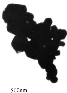
Figure 2. Transmission electron microscopy (TEM) micrograph of the sample: SnTe.
